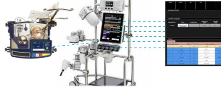
Connectivity feature: autoLog IQ data downloaded directly in the Quantum System Workstation
